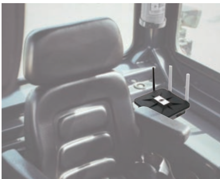
Place Cabin AP next to crane operator seat
